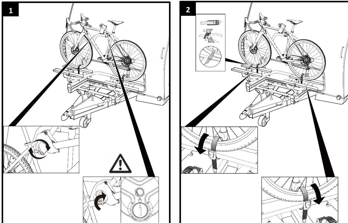
To prevent from any twisting, always double-tighten the front wheel of the bicycle using the supplied short textile strap.
